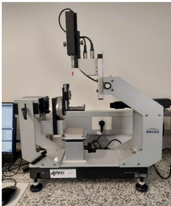
**Fig. 4.** The Drop Shape Analyzer by Krüss.
