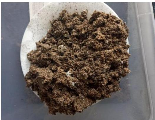
**Fig. 3.** Tanning shavings used in granulation (source: own research data)
