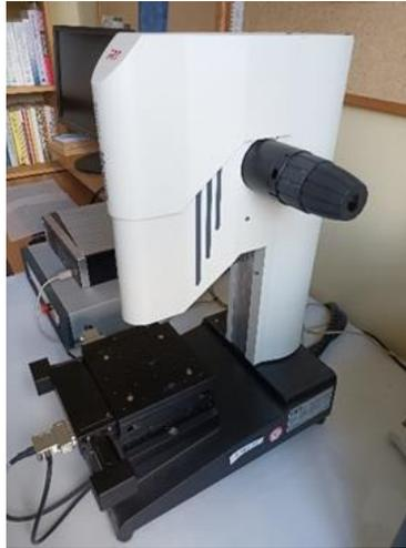
**Fig. 2.** MicroSpy® Profile profilometer by the FRT the art of metrology™.
