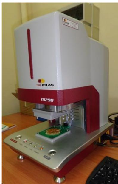
**Fig. 3.** The Moisture Management Tester M290 by SDL ATLAS (US).
