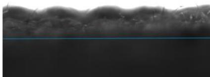
**Fig. 9.** View of sessile drop from measurement for twill 2/2 weave woven fabric.
