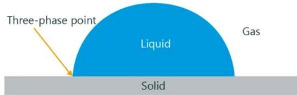
**Fig. 6.** Schematic diagram of a three-phase system
